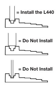
Determine the gap between the edge of the door and the cabinet frame by inserting the sizing tool between the edge of the door and the fixture frame where the L440 will be mounted, as far as it will go without forcing it. Read the number on the step that fits between the edge of the door and the cabinet frame.
