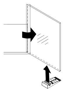
If the glass does not fit into the gauge or fits into the smallest groove do NOT install the L440.
