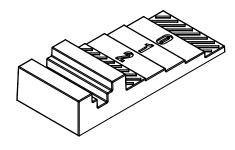
Open the glass door and hold the sizing tool against the edge of the glass.
