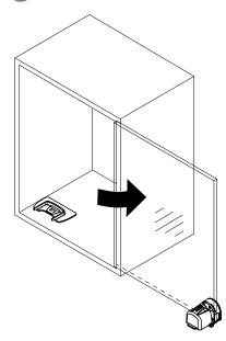
To lock the L440, shut the door and listen for the click to confirm that the L440 is locked.
