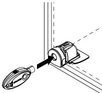
**Note:** If the key does not beep and makes a "knack-knack" sound it means the key was pulled away too soon. Try again and wait for the beep before pulling the key away.
