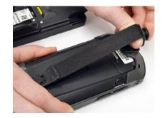
6 Unhook the top connector of the handstrap from the Zebra device.
