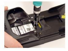
Reinsert and tighten the 4 screws.
