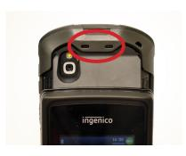
Ensure that the rubber exoskeleton on the Zebra device, hooks over the tabs on the case.
