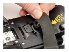
Attach the handstrap from the Zebra device to the connection point within the case.
