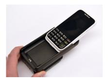
Slide the Verifone E285 into the side of the case with the USB-C connector.
