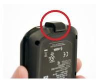
Ensure that the tabs on the connector snap into the slot on the TC20.
