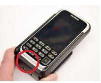
Ensure that the E285 is fully seated on the USB-C connector.
