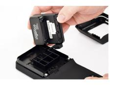
Plug the cable on the backside of the case into the card reader.
