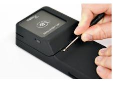
Slide the locking tab over to release the card reader cover from the case.
