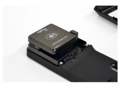
Place the card reader into the cavity in the case.
