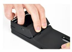
Grip the top portion of the card reader and apply pressure to separate the cover from the case.
