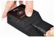
6 Slide the locking tab over to secure the cover to the case.
