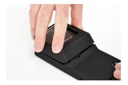
Fit the bottom edge of the card reader cover into the bottom of the case. Pivot the cover down over the card reader.
