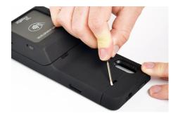
Slide the locking tab over to unlock the top cover on the case.
